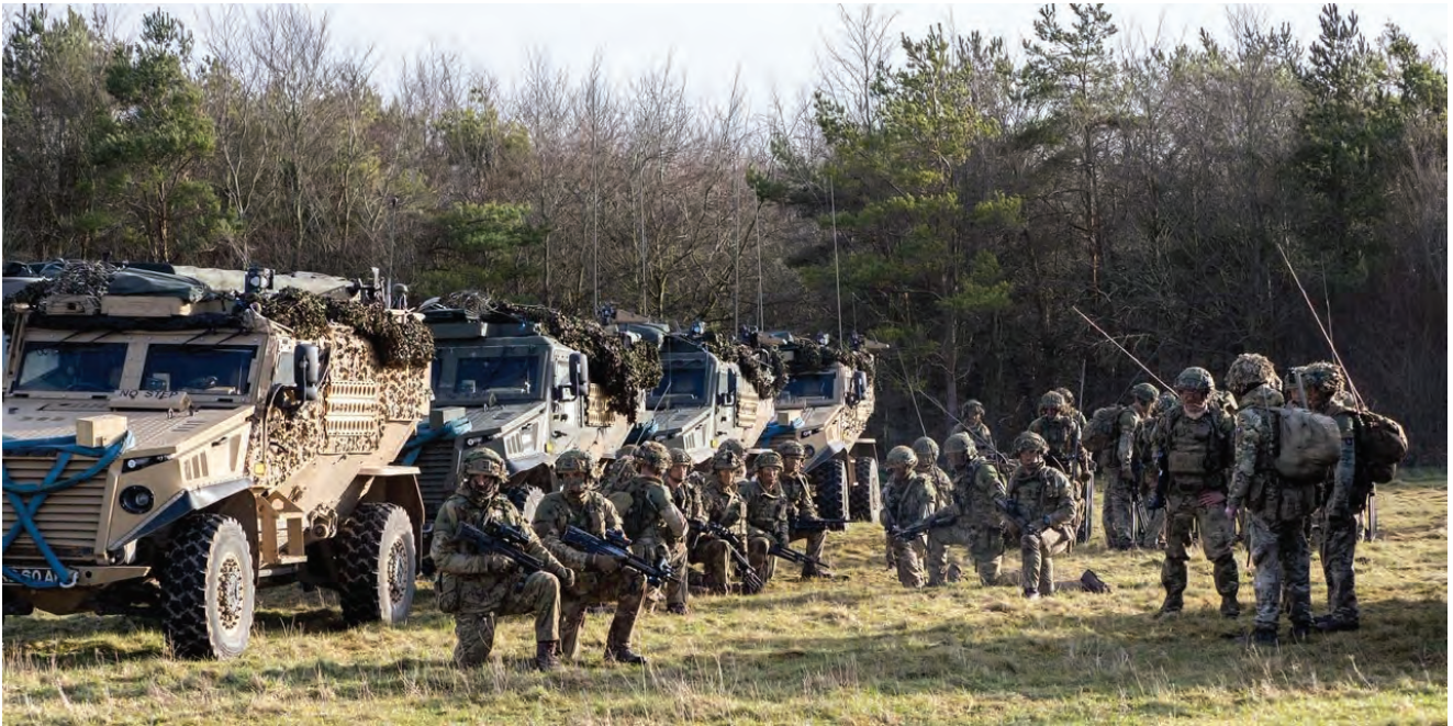
The workhorse of A (Lincolnshire) Company on Ex WESSEX STORM, the FOXHOUND protected mobility vehicle.
